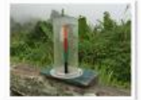
A rain gauge is used to measure the amount of rainfall.
